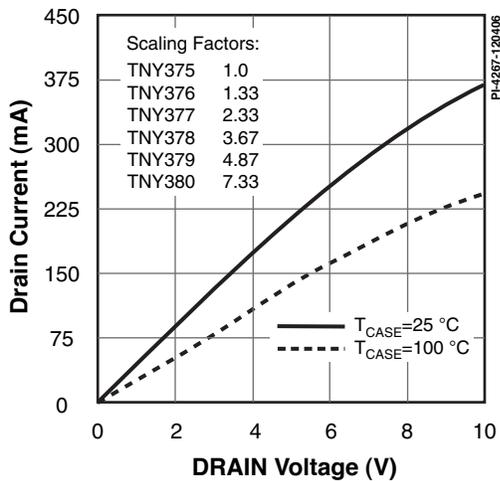
Figure 25. Output Characteristics.
