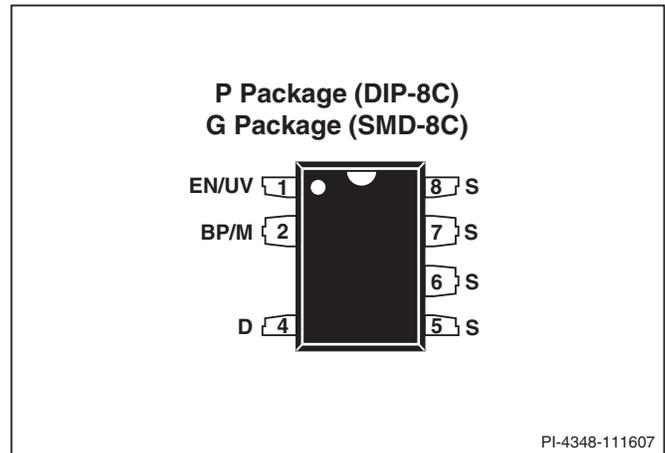
Figure 3. Pin Configuration.
