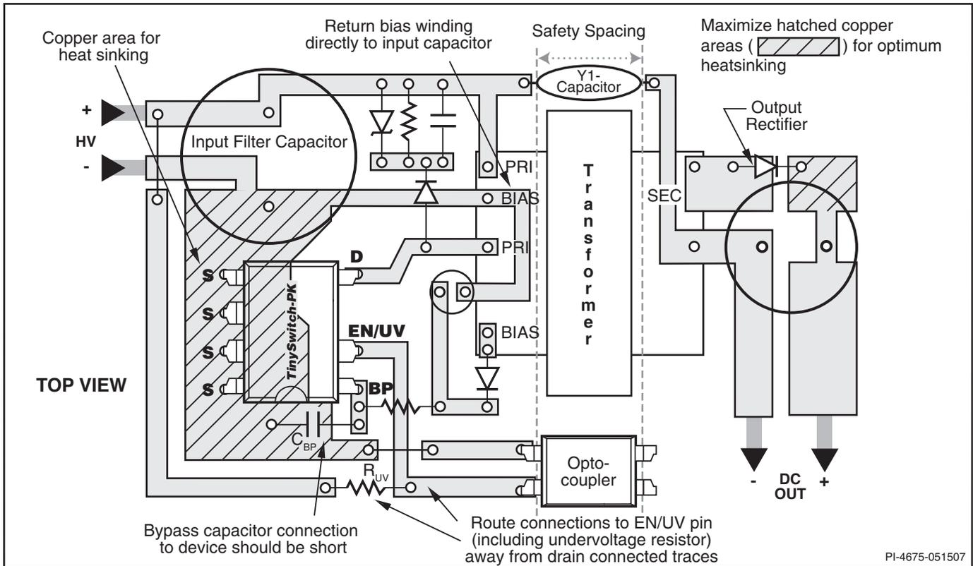
Figure 16. Layout Considerations for TinySwitch-PK Using P Package.
