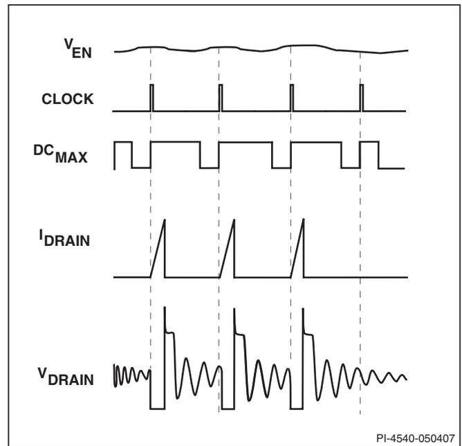
Figure 8. Operation at Medium Loading ( $f_{osc}$  132 kHz).
