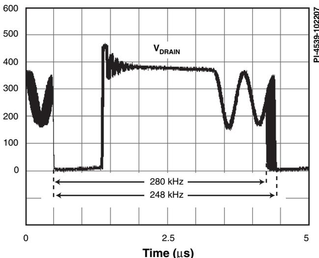
Figure 4. Frequency Jitter.
