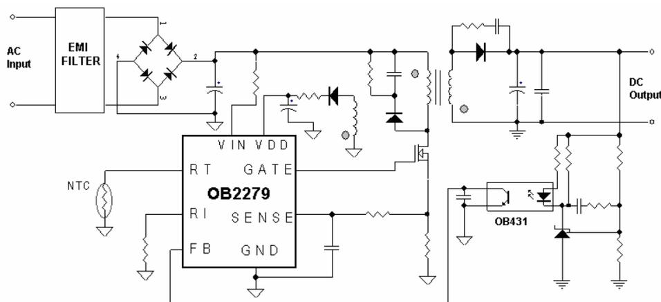
**Current Mode PWM Controller** Freq Shuffling with Latch Shutdown
