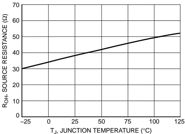
Figure 11. Output Source Resistance vs. Junction Temperature
