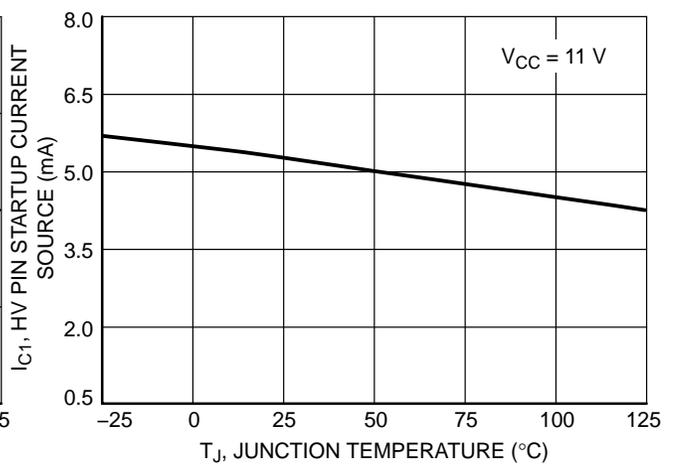
**Figure 8. HV Pin Startup Current Source vs. Junction Temperature**
