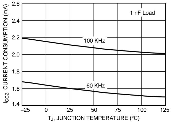
**Figure 6. IC Current Consumption, I<sub>CC2</sub> vs. Junction Temperature**
