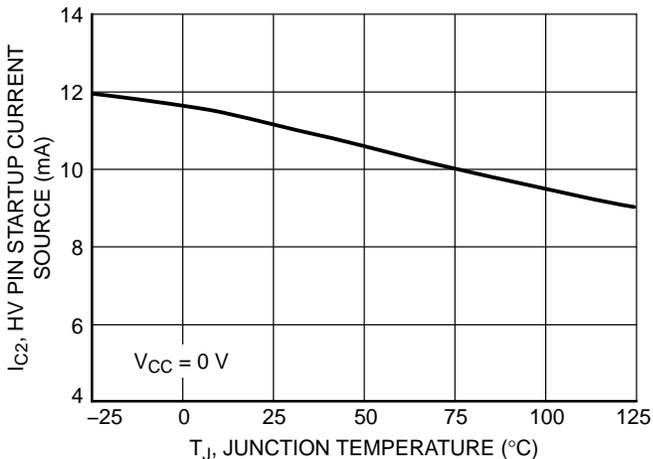
Figure 9. HV Pin Startup Current vs. Junction Temperature
