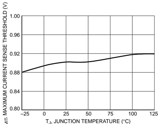
Figure 14. Maximum Current Sense Threshold vs. Junction Temperature
