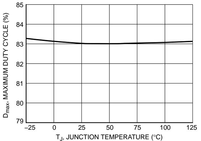
Figure 20. Maximum Duty Cycle vs. Junction Temperature
