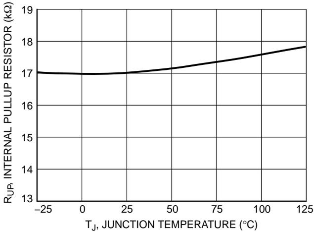
Figure 21. FB Pin Pullup Resistor vs. Junction Temperature
