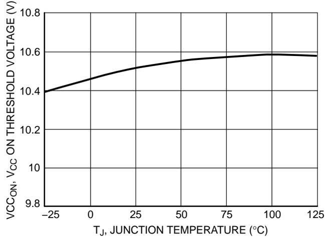
**Figure 4. V<sub>CC</sub> ON Threshold Voltage vs. Junction Temperature**
