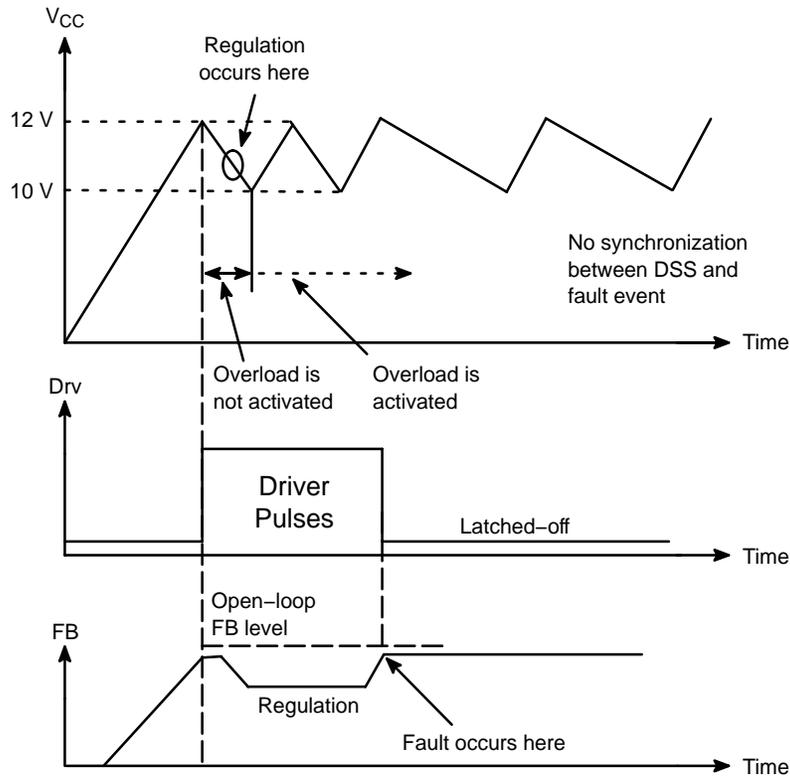
Figure 34. Fault Protection Timing Diagram
