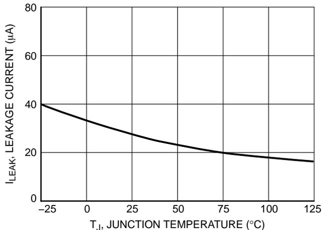
Figure 10. Leakage Current vs. Junction Temperature
