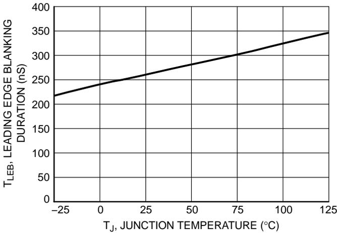
Figure 17. Leading Edge Blanking Duration vs. Junction Temperature
