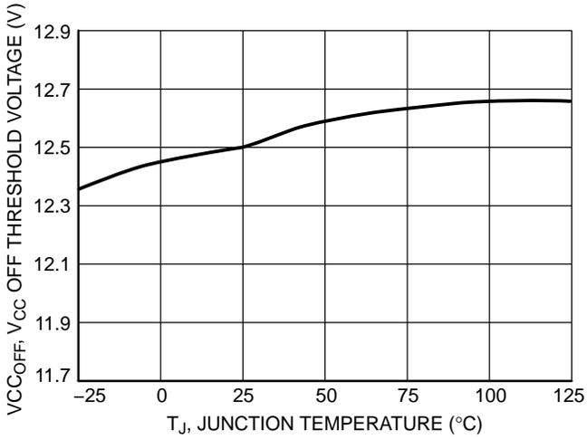
**Figure 3. V<sub>CC</sub> OFF Threshold Voltage vs. Junction Temperature**
