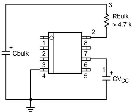
**Figure 36. A simple resistor in series avoids any latchup in the controller**
