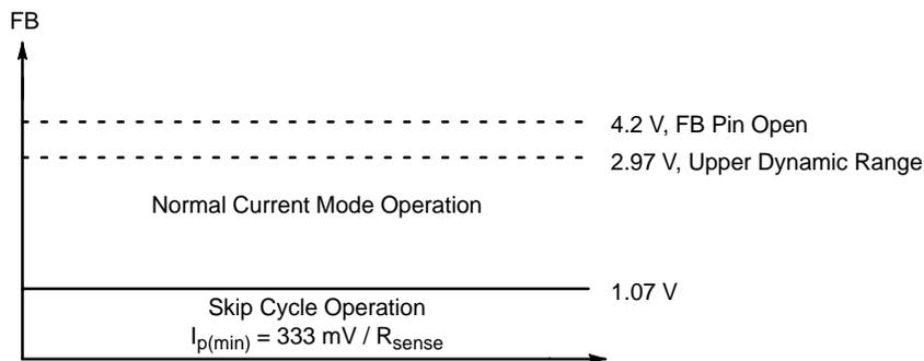
**Figure 29. Feedback Pin Voltage and Modes of Operation**
