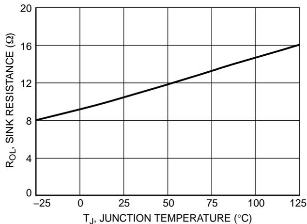
Figure 12. Output Sink Resistance vs. Junction Temperature
