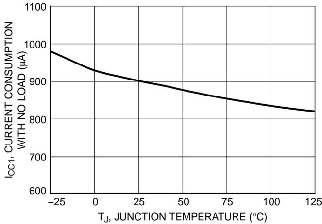
**Figure 5. IC Current Consumption, I<sub>CC1</sub> vs. Junction Temperature**
