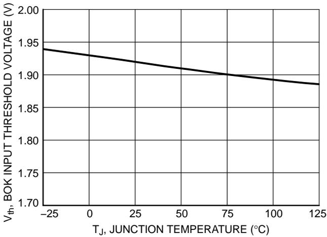
Figure 23. BOK Threshold Voltage vs. Junction Temperature
