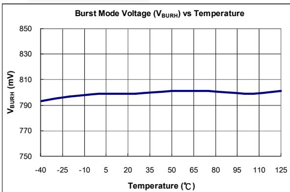
**Figure 8. Burst-Mode Voltage ( $V_{BURH}$ ) vs. Temperature**
