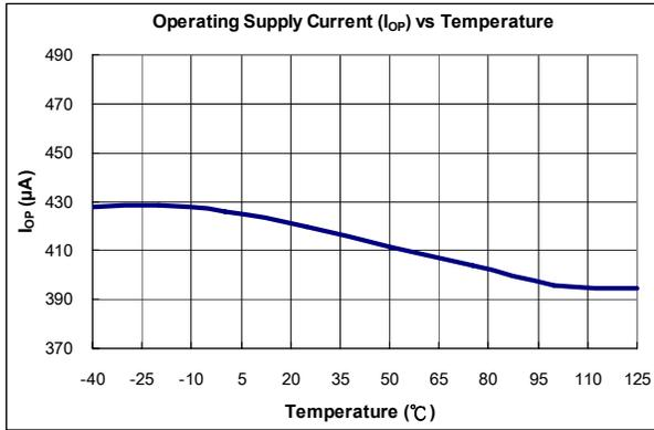
**Figure 4. Operating Supply Current ( $I_{OP\_Burst}$ ) vs. Temperature**
