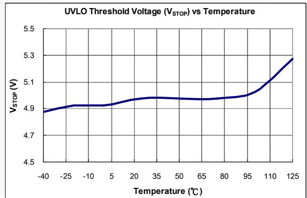
**Figure 7. UVLO Threshold Voltage ( $V_{STOP}$ ) vs. Temperature**
