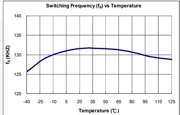
**Figure 5. Switching Frequency ( $f_s$ ) vs. Temperature**
