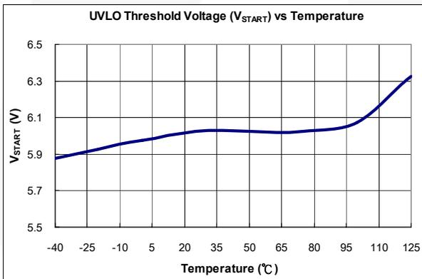
**Figure 6. UVLO Threshold Voltage ( $V_{START}$ ) vs. Temperature**
