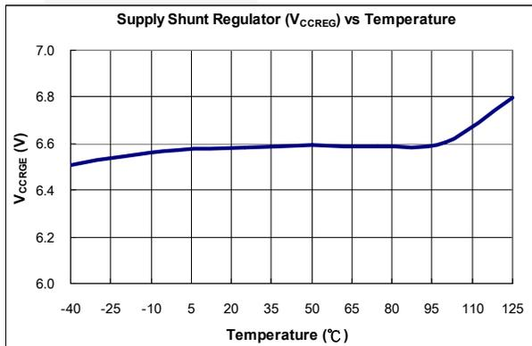
Figure 14. Supply Shunt Regulator ( $V_{CCREG}$ ) vs. Temperature
