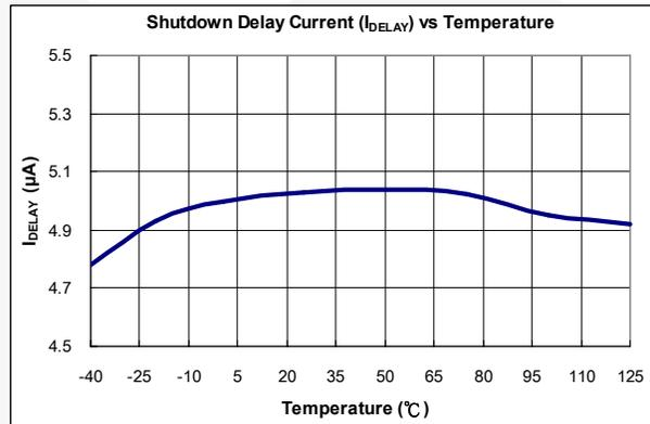
Figure 13. Shutdown Delay Current ( $I_{DELAY}$ ) vs. Temperature
