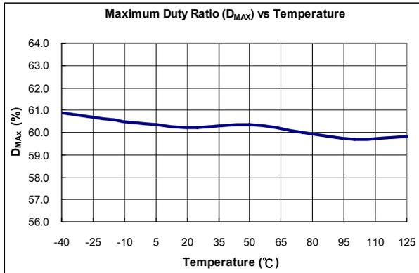
Figure 10. Maximum Duty Ratio ( $D_{MAX}$ ) vs. Temperature
