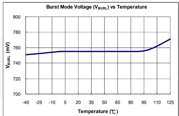
**Figure 9. Burst-Mode Voltage ( $V_{BURL}$ ) vs. Temperature**
