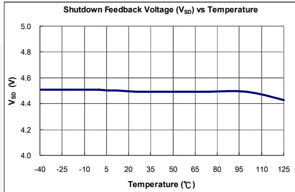
Figure 11. Shutdown Feedback Voltage ( $V_{SD}$ ) vs. Temperature
