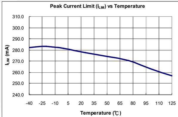
Figure 12. Peak Current Limit ( $I_{LIM}$ ) vs. Temperature
