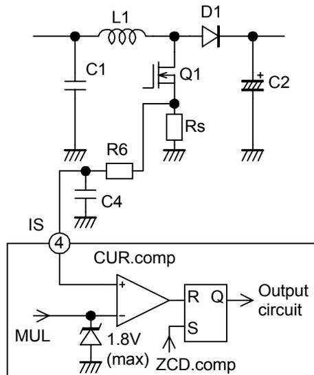
Fig.8 Current sense comparator circuit
