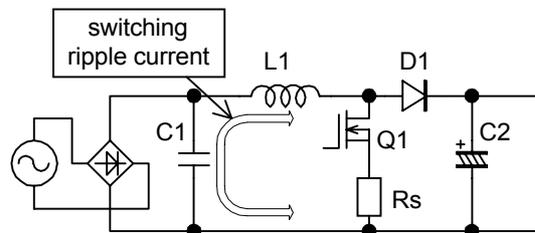
Fig.27 Input capacitor circuit
