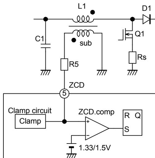
Fig.9 ZCD circuit
