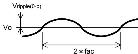
Fig.28 Output ripple voltage
