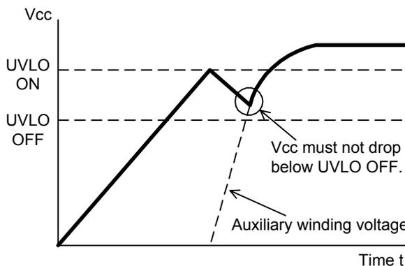
Fig.20 Vcc voltage at startup
