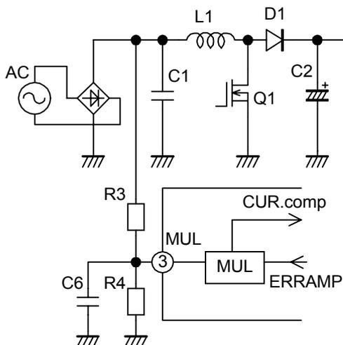
Fig.7 Multiplier circuit
