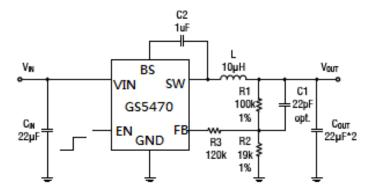
Figure 1. Basic Application Circuit
