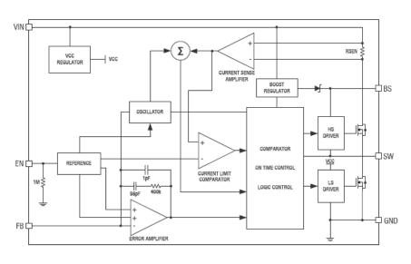
Figure 2. GS5470 Block Diagram
